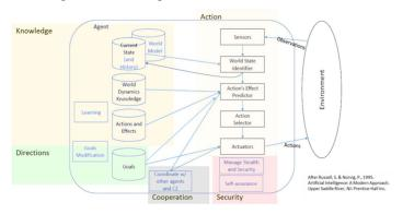
Figure 1 Assumed functional architecture of the AICA
